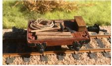
Whilst these wagons were useful, a cheaper alternative was also investigated in the form of a 3d printed chassis from Locos n stuff at about £6 each. These needed a bit of cleaning up and Jürgen found that half a Peco coach side fitted nicely to these chassis. This made a small, single comparment coach full of character and ideal for his compact layouts.
