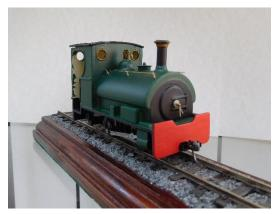
One of my lockdown projects has been to complete an 016.5 0-4-0 saddle tank loco built from a Smallbrook Studio body kit on a Hornby Ben chassis. I've had two of these kits for about 5 years or more and
