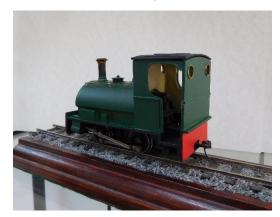
face smokebox door though. I also added extra detail to the body with a Branchlines brass smokebox door dart and also regulator handle, hand brake and reversing lever in the cab from the same source.
