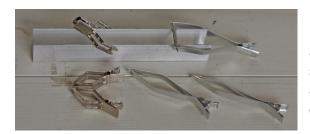
It is a very simple jig designed and manufactured by Frank Sharp on behalf of the 7mm NGA. The main part is a length of 20mm aluminium channel with accurately machined 'V' notches in each side of the channel. These locate one of the 1/8 inch diameter axles which have pointed ends on which you can locate the coupling rods.
