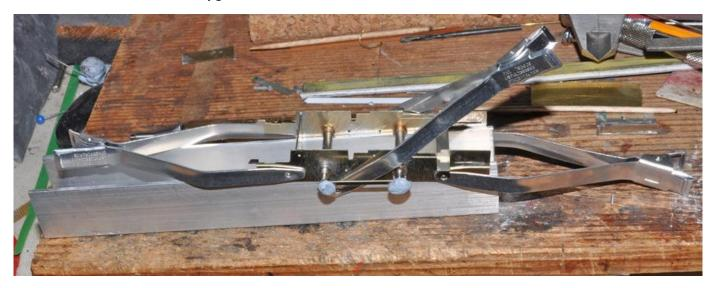
Setting it up proved quite straightforward and I used the long clamps to hold the chassis sides in position as they gave more access for the soldering iron. With the channel holding the sides the correct width it was quite easy to use longer metal strips through some of the chassis spacer slots and additional spacers were added once the basic shape had been secured.
