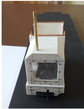
It is based on a Lister diesel and is modelled to Gn15. The chassis used is a Hornby Smokey Joe which he had lying around. Most of the construction is from Plasticard with other bits and pieces out of the scrap box.
