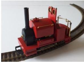
Regular contributor Dave has just completed this locomotive which has been built from a Smallbrook Studio kit (Gn15 body kit) and is called 'Harlequin'. Mainly built as intended but with a few modifications. The resin whistle has been changed to a homemade brass one and the gauge (part of the resin back plate) has been changed to a brass one. The chassis is from a second hand Hornby Smokey Joe.
