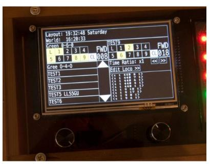
At the top is the actual time and the layout time that is saved when the controller is turned off. Time can also be sped up by touching the Time ratio buttons on screen.
