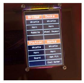
The sounds for these will play from small speakers mounted into various positions on the layout. The four headings are the four boards so it makes sure when a background sound is selected it plays on the correct board.
